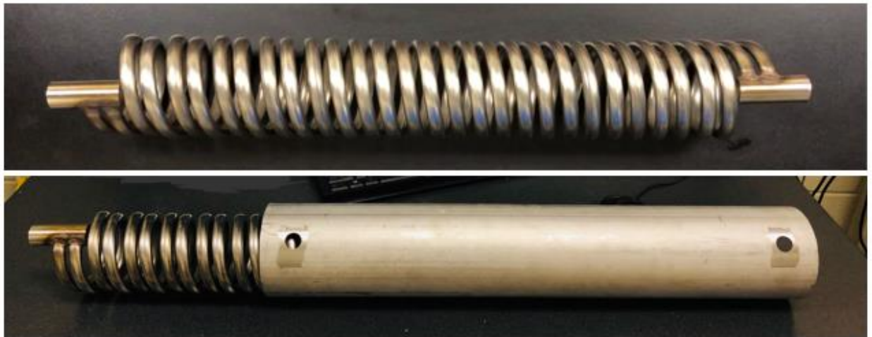
Figure 8 Picture of the double helically coiled heat exchanger without and with the secondary coolant shell
