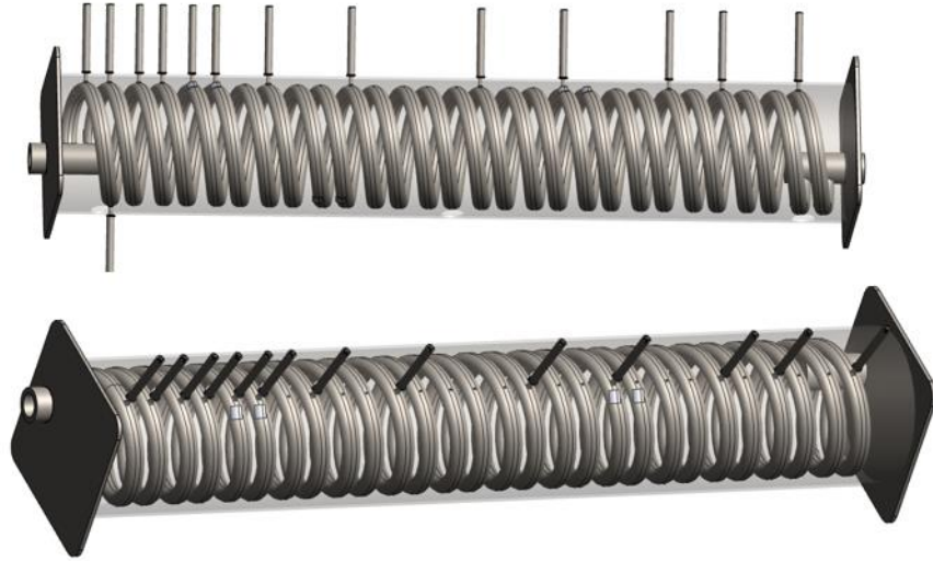
Figure 80 Placement of thermocouples on both the primary and secondary side
