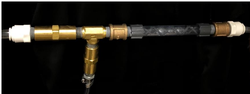
Figure 13 T-section and inline static mixture use to mix the air and water
