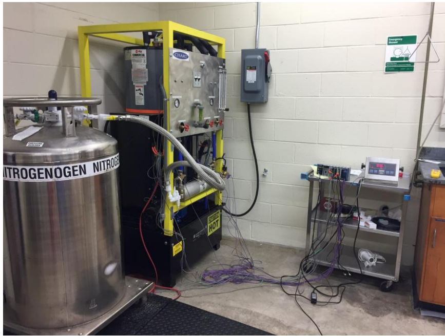
Figure 9 Lab setup to test the double helical heat exchanger using Liquefied Nitrogen Gas (LN2)
