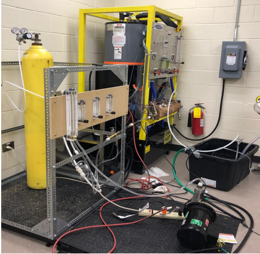
Figure 11 Lab setup to test the hydrodynamic characteristics of a gas-liquid two-phase flow using air and water
