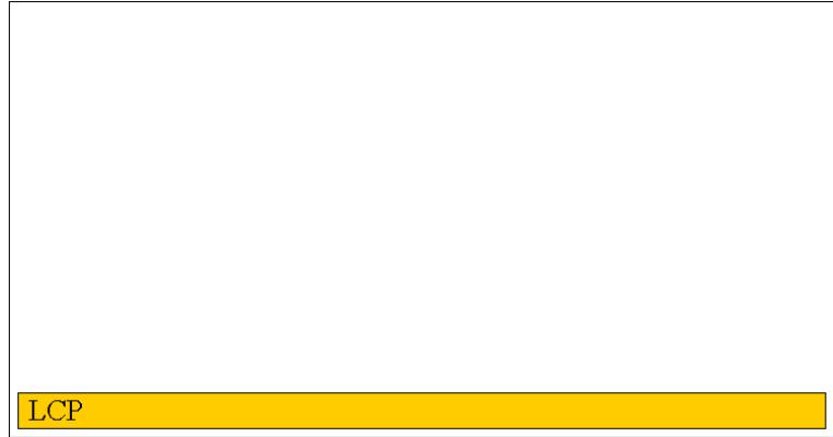
Figure 7: Fabrication starts with a clean, smooth, bare LCP wafer
