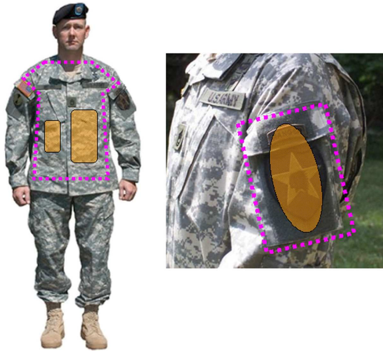
Figure 138: A wearable antenna system is shown. The communication device is sewn directly into the soldier's uniform. Potential areas for integration are outlined in pink. The areas in orange denote convenient areas to place sensors to detect vital signs.
