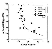
Fig. 5 The correlation between the relative kappa number reduction through hydrolysis and the pulp kappa number for five North American hardwood pulps.
