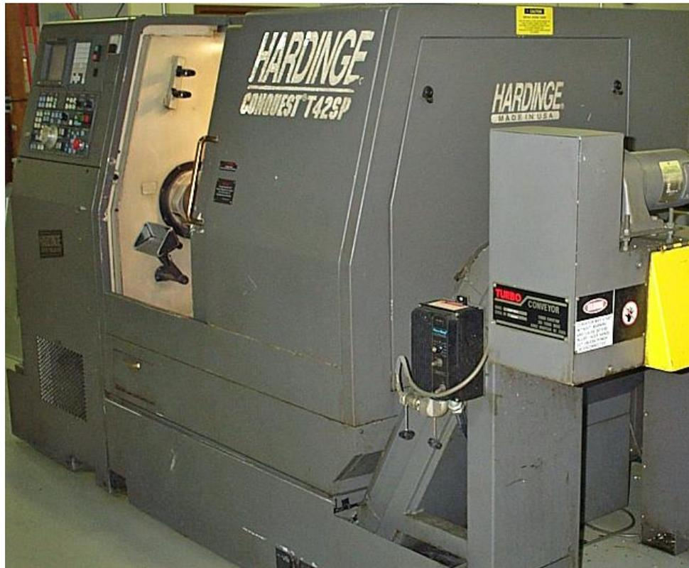
**Figure 8.1.5:** Hardinge Conquest CNC lathe [courtesy: Hardinge Inc.].
