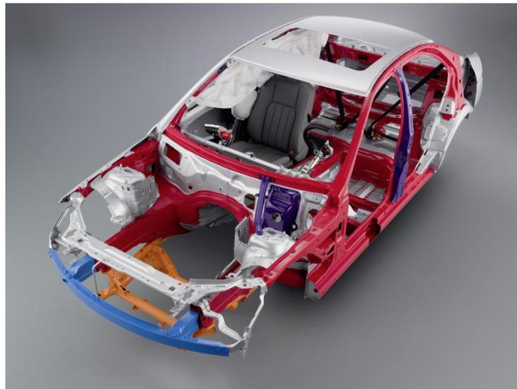
**Figure 1.2:** High strength steel structure in Mercedes-Benz passenger car
