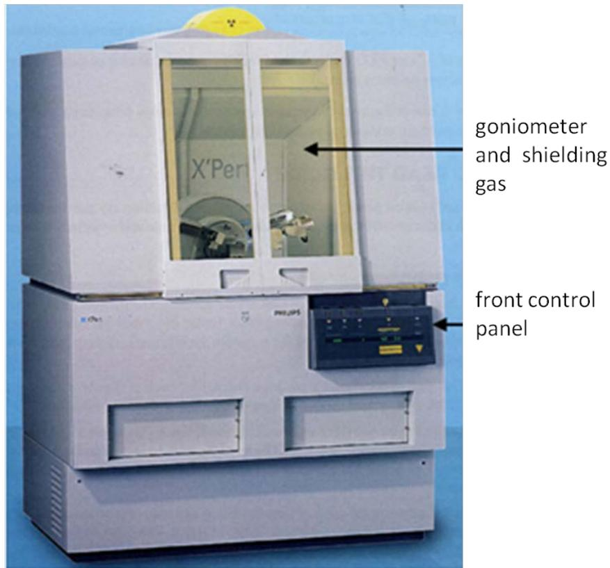
**Figure 8.3.3:** PANalytical X'Pert Pro MPD [courtesy: PANalytical].
