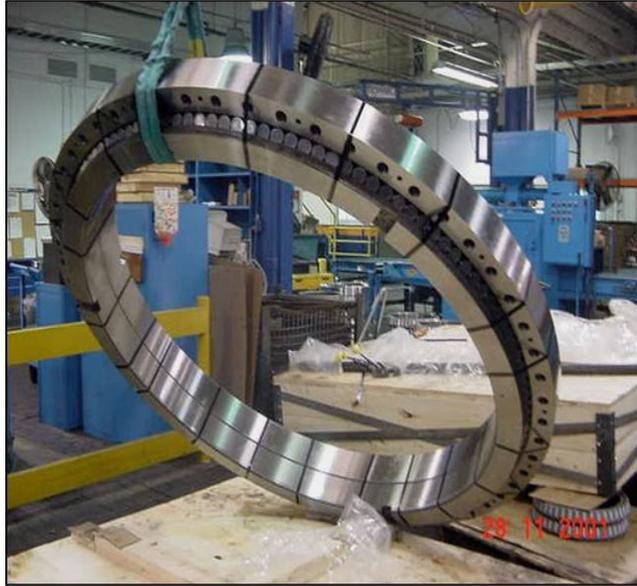
**Figure 1.3:** Large bearings for wind turbine [courtesy: The Timken Company].
