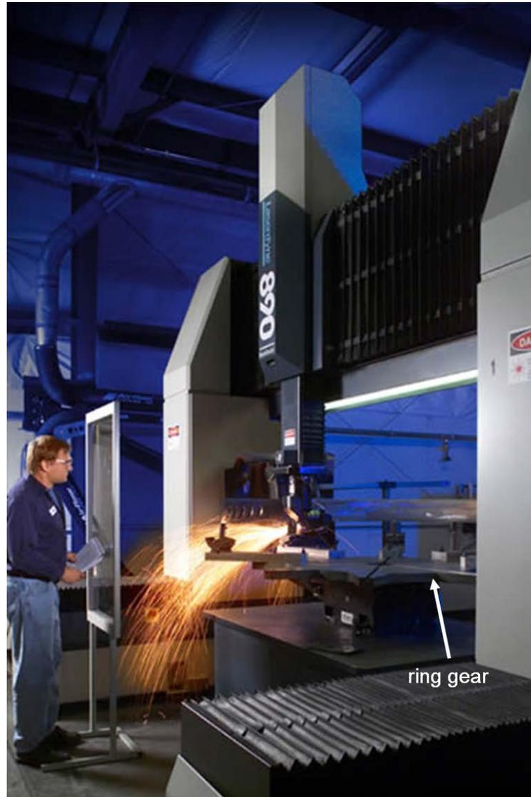
**Figure 2.13:** Five-axis laser machining center precision processes a ring used in a power-generation turbine [courtesy: LAI International].
