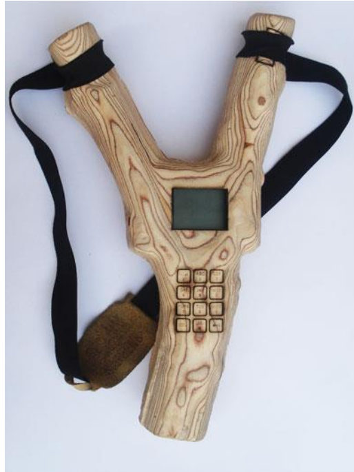
Figure 16 – Users key a message using the keypad then aim and fire the slingshot at the wall. (Fischer, Hornecker, and Zoellner 2013).
