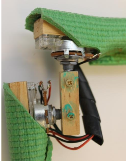
Figure 30 – The shoulder joint of the puppet with potentiometers mounted perpendicularly to allow a full range of motion in the x, y, and z planes.
