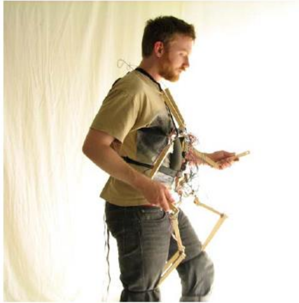
Figure 29 – The BDC puppet, a hybrid full-body/rod puppet that balances ease of use and expressivity to track full body movement of the puppeteer.
