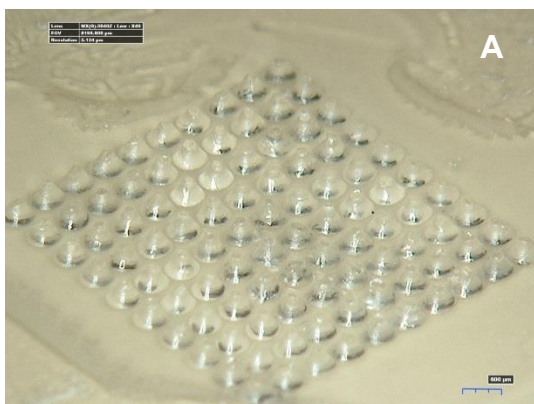
Figure C.2 Volume of microneedle dissolved and representative images of microneedles between one click and five clicks.
