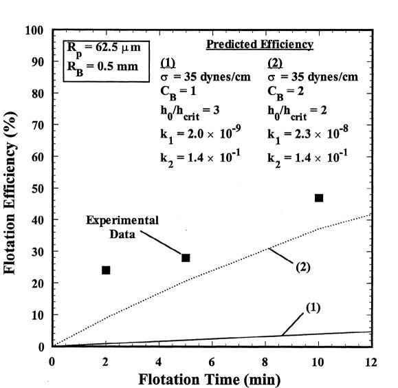
Figure 12: Experimental and theoretical flotation removal efficiency for  $R_p = 62.5 \ \mu \text{m}$  and  $R_B = 0.5 \ \text{mm}$ .
