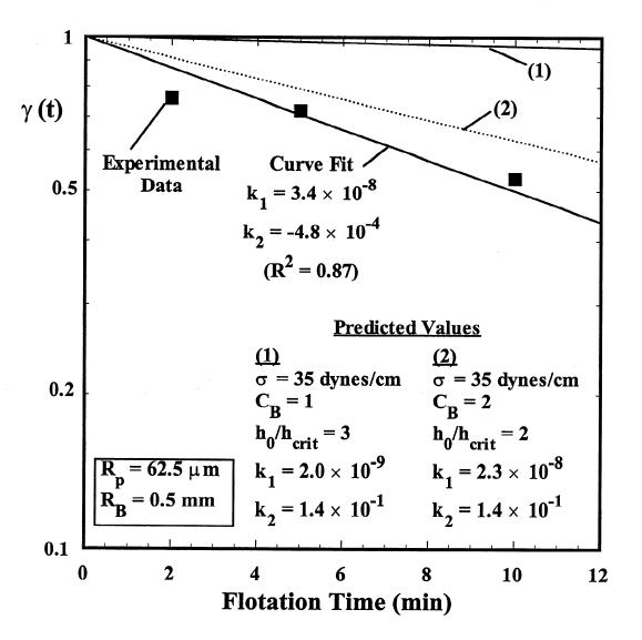
Figure 11: Experimental and theoretical  $\gamma(t)$  for  $R_p = 62.5 \mu \text{m}$  and  $R_B = 0.5 \text{ mm}$ .
