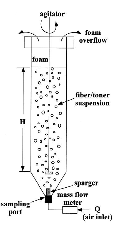
Figure 1: Schematic of the laboratory flotation cell used in this study.
