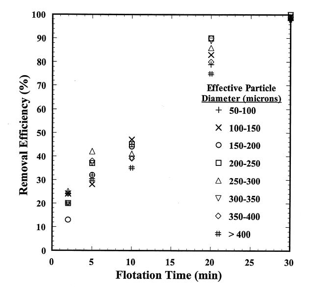
Figure 10: Average removal efficiency as a function of flotation time for different particle size ranges.
