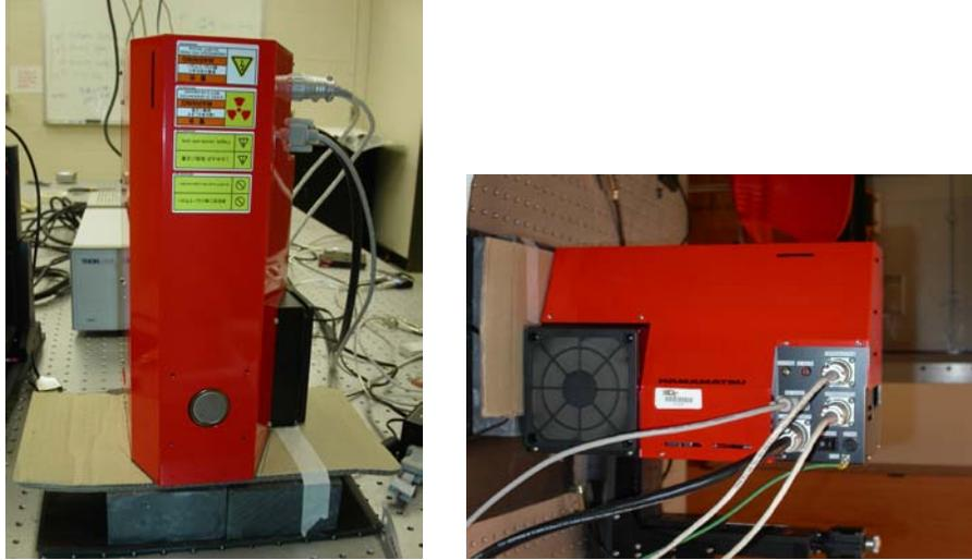
Figure 2.2: Hamamatsu L9631 Micro-Focus X-ray Source
