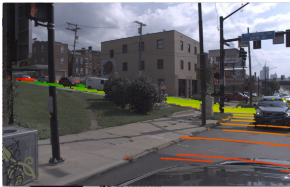
Figure B.1: A scene with non-planar ground surface. The colored LiDAR returns have been classified as belonging to the ground, based on the map. Points outside the driveable area are also discarded. This simple distance threshold against a map works well, even on the road to the left which goes steeply uphill.
