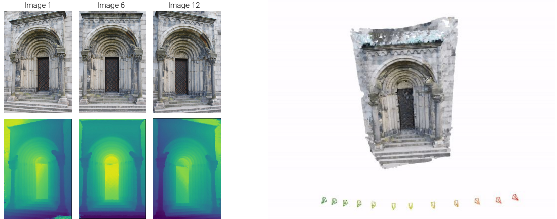
Figure 3.13: Qualitative results of GTSFM on the Lund Door dataset, consisting of 12 images. (Left) Depth maps, generated by PatchmatchNet [215]. (Right) Multi-view stereo output (aggregation of backprojected depth maps).
