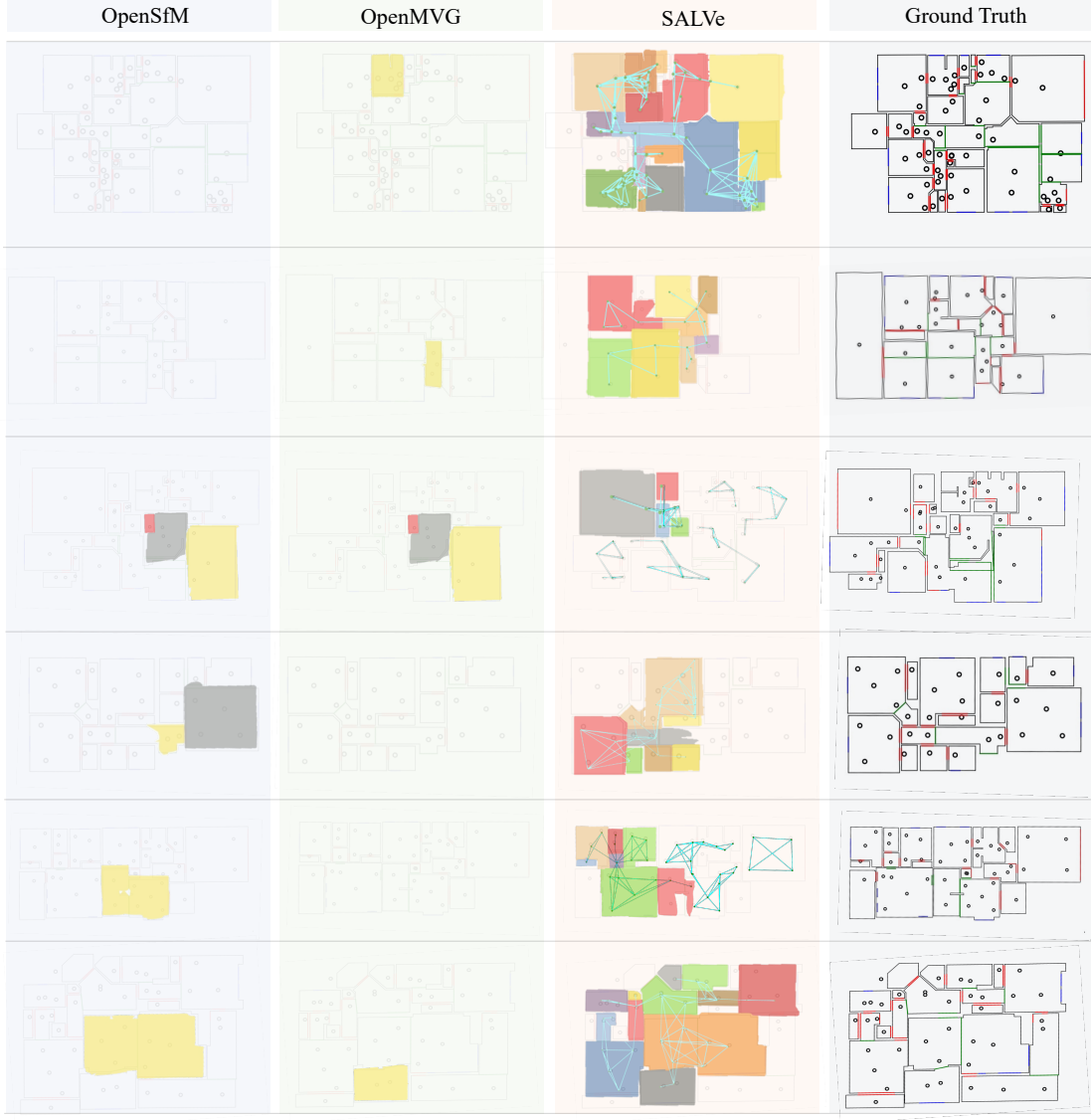
Figure 2.7: Qualitative comparison of floorplan results. Column 1: OpenSfM. Column 2: OpenMVG. Column 3: Ours. Column 4: Ground truth floorplan. All results are superimposed on the ground truth floorplan. Colored regions indicated the reconstruction result; at times, the baselines localize no panos. Our floorplan recall is significantly better than the state-of-the-art. Each row corresponds to a single floor of a different home. Colored lines represent W/D/O objects – doors , openings and windows . The multiple cyan edges in the overlaid graph correspond to verified W/D/O alignment hypotheses. For an open layout, a successful case often involves edges from panoramas in many different rooms to a single pano. These examples are intended to offer an even-handed selection of reconstructions that indicate both good performance as well as areas for improvements. Rows 1 and 6 illustrate good reconstructions. Row 2 illustrates a more challenging case with only 1-2 panos in most rooms. Rows 3-5 are more challenging as they include bottlenecks in the actual physical layout, which is critical in joining connected components.
