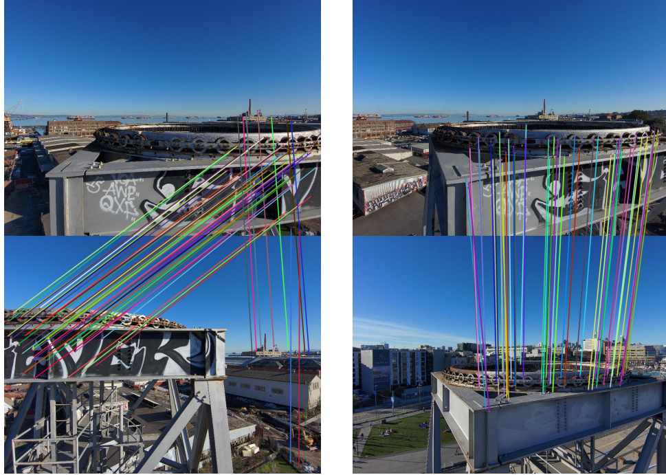
Figure 1.4: Examples of good ( left ) and poor ( right ) matches from a deep feature detector/descriptor (SuperPoint [42]) and deep matcher (SuperGlue [76]) for two image pairs, from Skydio’s Crane Mast dataset. False positives ( right ) occur because of repetitive structures.
