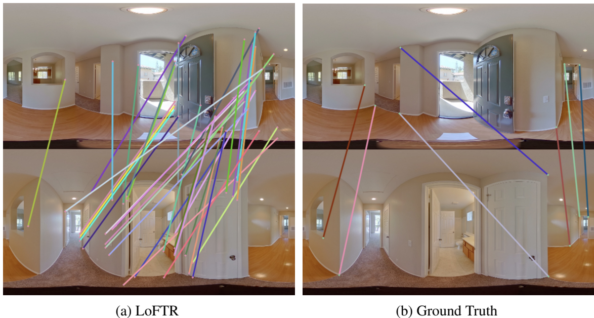
Figure 5.3: (Left) : 50 most confident keypoint matches from LoFTR [82], a state-of-the-art image matching system, on an image pair from ZInD [14]. (Right) : Ground-truth (hand-annotated) keypoint matches for the same image pair. 50 out of 50 LoFTR matches are incorrect, each with estimated confidence over 0.9.
