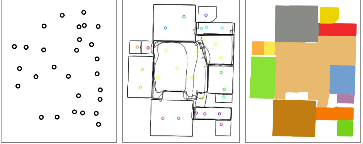
Figure 2.4: An example of different stages of floorplan reconstruction: Left : Estimated positions of panorama centers. Center : Grouped panoramas with estimated dense room layouts. Panorama centers with the same color are part of the same group. Notice that each open space is grouped together. Distinct groups correspond largely to physical rooms separated by doors. Right : The final floorplan after highest-confidence contour extraction is applied to each group. Each contour is filled with a unique color.
