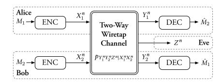
FIGURE 3.2 – Communication over a two-way wiretap channel without feedback.
