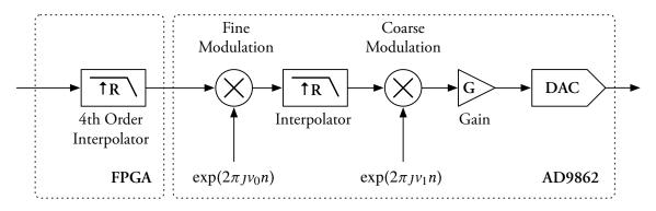
FIGURE 7.5 – Signal modulation and transmission.
