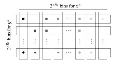
**FIGURE 2.6** – Binning procedure for the Slepian-Wolf coding. Each pictogram represents one of the  $2^{n\mathbb{H}(XY)}$  jointly typical pairs  $(x^n, y^n)$ .
