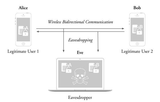
FIGURE 1.4 – Simple multi-user scheme with eavesdropper.
