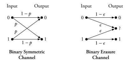
FIGURE 2.3 – Binary symmetric channel and binary erasure channel.
