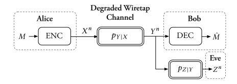
**FIGURE 1.1** – Communications over the degraded wiretap channel.
