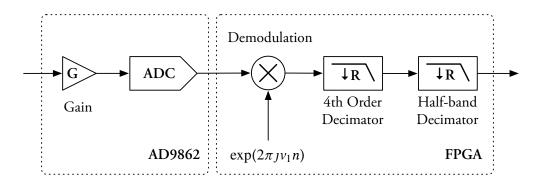
FIGURE 7.6 – Signal reception and demodulation.
