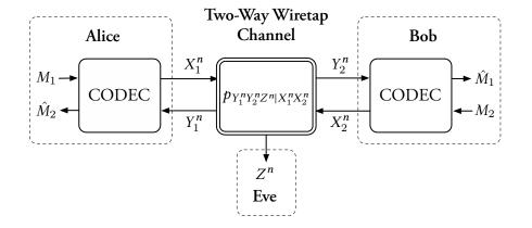
FIGURE 3.1 – Communication over a two-way wiretap channel.
