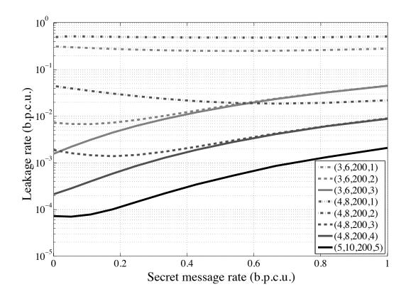
**FIGURE 5.4** – Leakage v.s. communication rate for various codes and puncturing rates. Codes with w = 1 correspond to classical LDPC codes.
