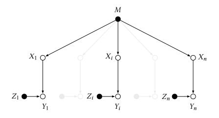
**FIGURE 2.1** – Functional dependence graph of Example 2.1.5. Independent random variables are indicated by  $\bullet$ , while functions of these random variables are indicated by  $\circ$ .
