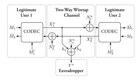
FIGURE 5.1 – Communications over the Gaussian two-way wiretap channel.
