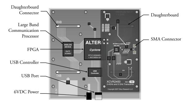
FIGURE 7.2 – Overview of a software-defined radio (USRP1).
