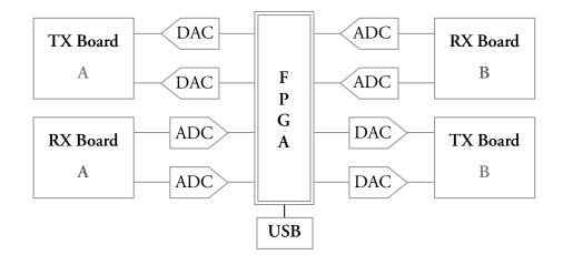
FIGURE 7.3 – General diagram of a software-defined radio.
