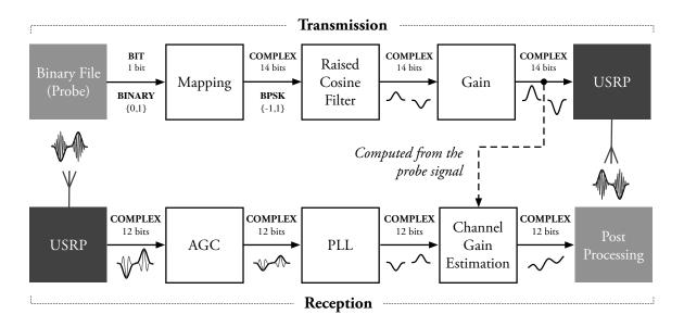
FIGURE 4.2 – Communication chain for channel gain estimation.
