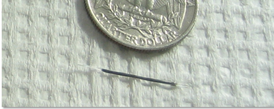
Figure 19: Permanently implantable electrode design consists of two Teflon coated silver electrodes bonded with epoxy. The hooked end is implanted around the ventral nerve cord and the opposing end protrudes from the dorsal integument of the cricket.
