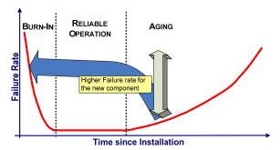
Fig. 5: Example of actions / diagnostics that produce too many Burn-Infailures.
