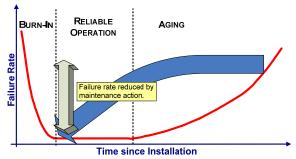
Fig. 3: Effect of diagnostic program when program was implemented at the correct time and sufficient actions can be deployed.
