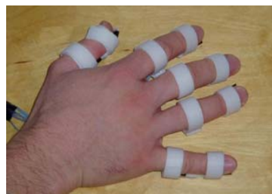
Figure 1 Sensor-based MIDI response device
