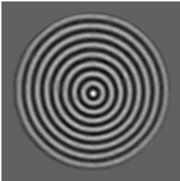
Figure 6.1: An axisymmetric target pattern is observed in our convection cell near onset (cell aspect ratio \Gamma = 20 , and \epsilon = 0.10 ).
