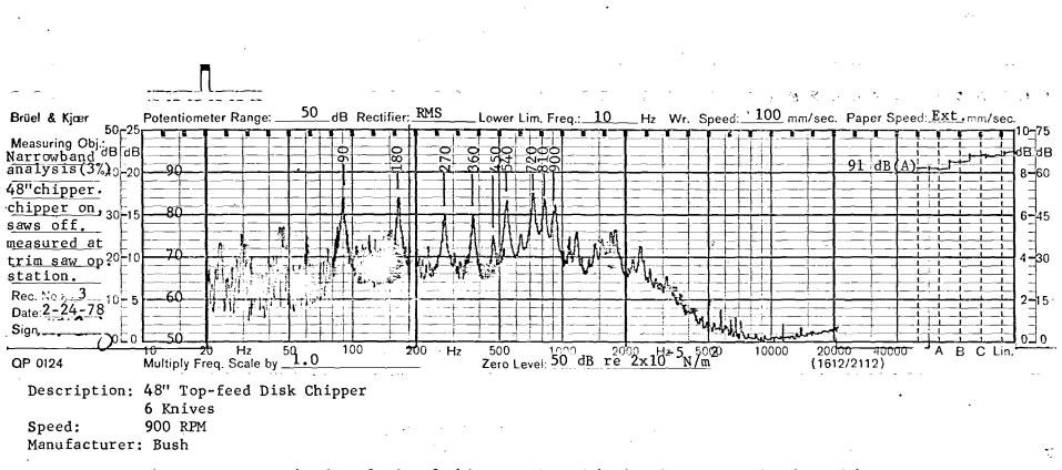
This is a narrow band analysis of chipper noise with the chipper running but with no wood going into the chipper. Measurement was made at the trim saw operator station.
