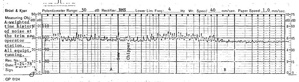
Time history of the A-weighted noise measured at the trim saw operator station. The zero level of the record equals 70dB re  $2x10^{-5}$  N/m<sup>2</sup>.
