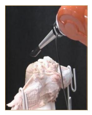
Initial work focused on developing a testcell to support studies on innovative automation cutting techniques. The cell constructed consists of a research robot, a variety of cutting end-effectors, a miniature force-torque sensor, and an array of digital cameras. In addition, the design team developed a computer model that incorporates measured cutting trajectories used by skilled workers to debone a chicken breast.
