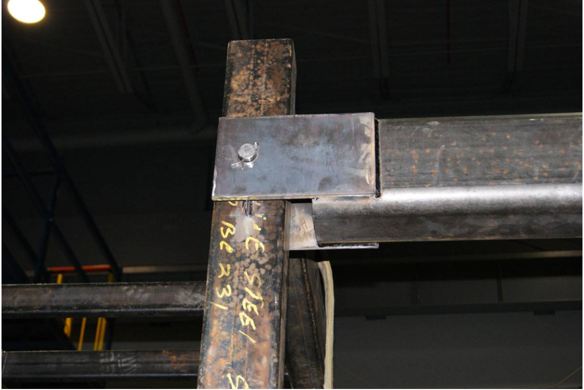
Figure 6.9: Pin connection for mass plate support beams for 1/10 th scale model
