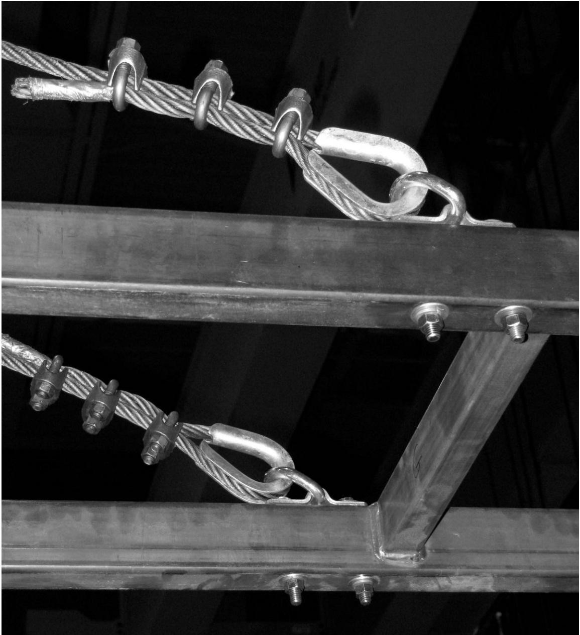
Figure 3.5: Stay connection detail for 1/20 th scale model
