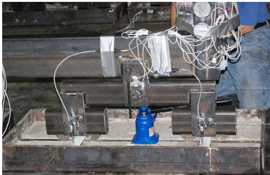
Figure 6.5: Photograph of boundary conditions for the 1/10 th scale model crane
