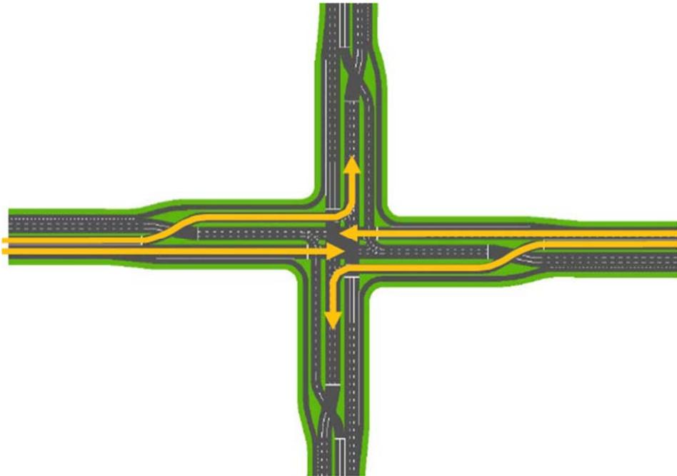
Figure 22. Continuous Flow Intersection Diagram.
