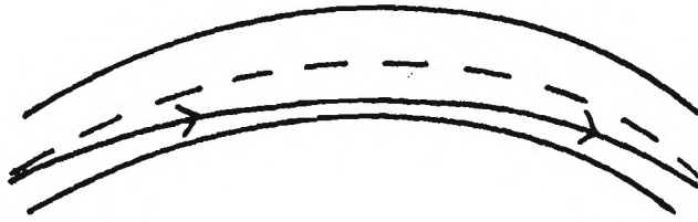
Figure 5. Illustration of a Cursor Path Which Minimizes Control Stick Manipulation at Expense of Position Error
