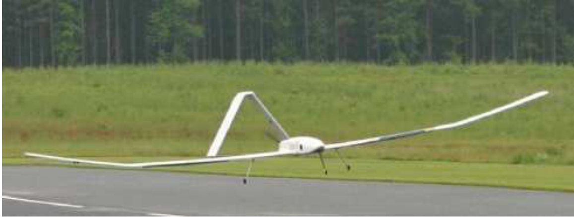
Figure 63. Fuel cell powered aircraft constructed for validation of design methodology
