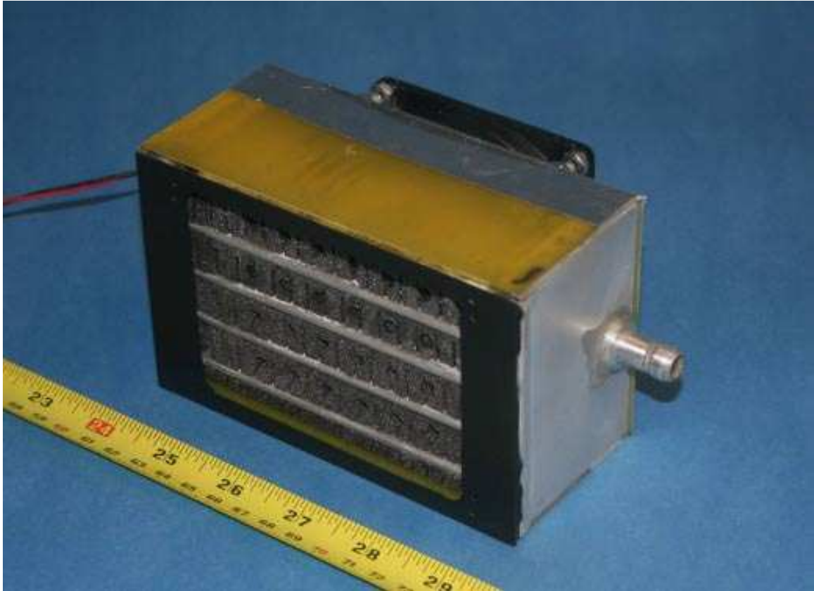
Figure 67. Carbon foam radiator as implemented in demonstrator aircraft
