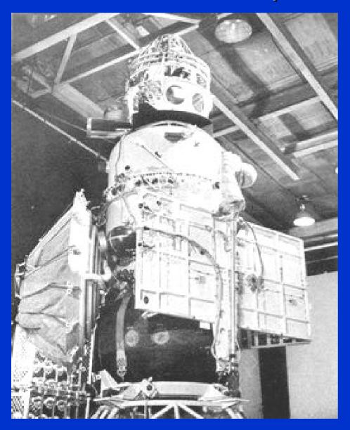
Venera 4 (1967) was the first soft entry probe; direct measurements at 55 to 23 km (18 bar)
