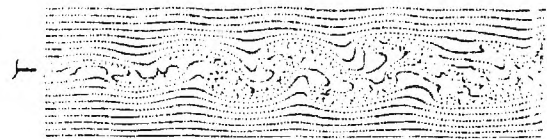
Figure 3. Wake Roll-up Behind a Flat Plate
