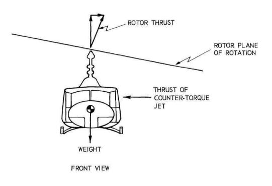
Fig. 8 Resultant Control Cross-Coupling
