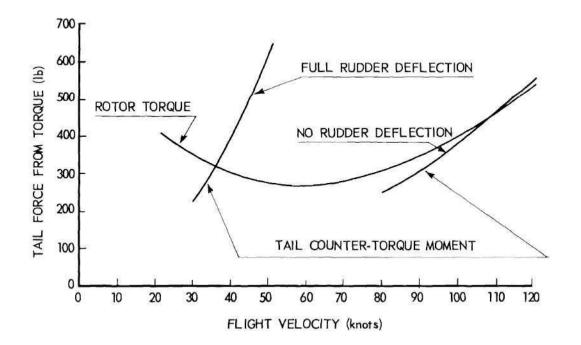
Fig. 3 Torque and Counter-Torque Forces Versus Flight Velocity
