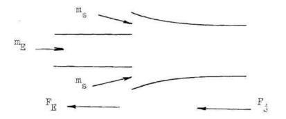
$m_E = mass flow of exhaust$   $F_E = thrust of exhaust$  $m_s = mass flow of secondary air$   $F_i = augmented thrust$
