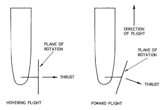
Fig. 1 Counter-Torque Rotor Incidence Due to Flapping
