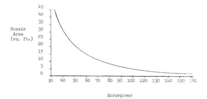
Fig. 5 Horsepower Variation with Nozzle Area
