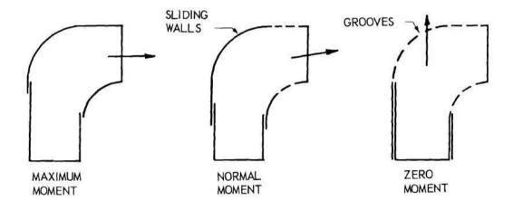
Fig. 7 Controllable Thrust Turning Elbow
