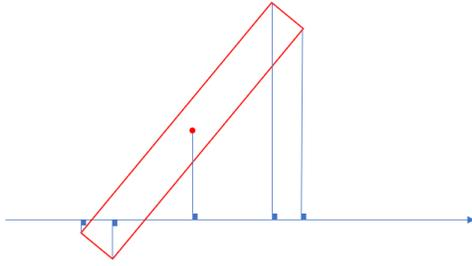
Figure 5: Illustration of the points of closest approach between a polygon with zero velocity and an object moving along the direction of the arrow
