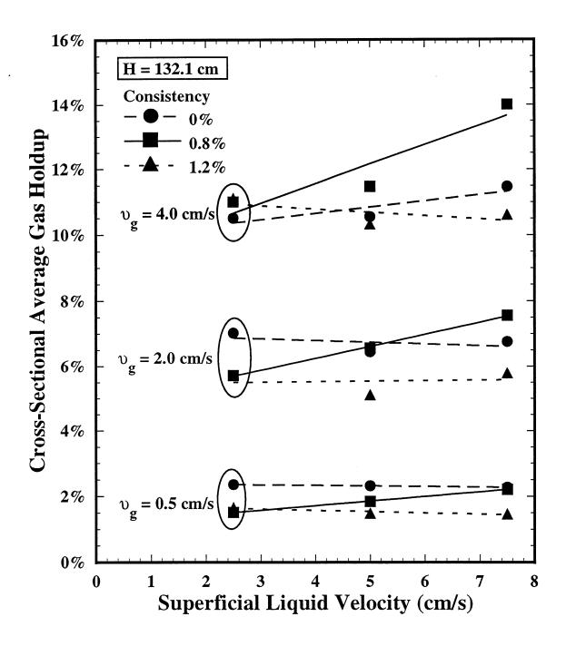
Figure 7: Cross-sectional average gas holdup as a function of superficial liquid velocity at H = 132.1 cm.
