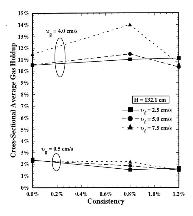
Figure 10: Cross-sectional average gas holdup as a function of ONP consistency at H = 132.1 cm.
