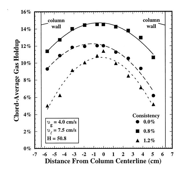
Figure 8: Chord-average gas holdup profiles at three different ONP consistencies for  $v_g$  = 4.0 cm/s,  $v_\ell$  = 7.5 cm/s, and H = 50.8 cm.
