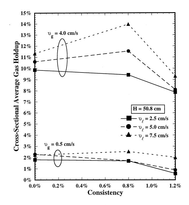
Figure 9: Cross-sectional average gas holdup as a function of ONP consistency at H = 50.8 cm.
