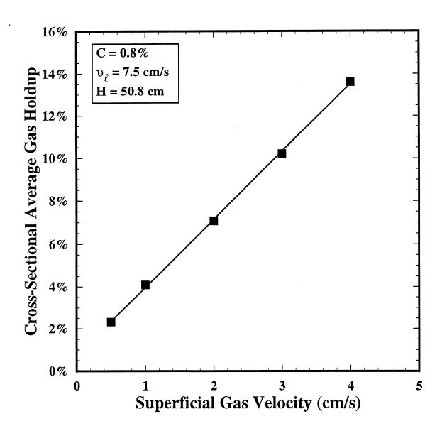
Figure 5: Cross-sectional average gas holdup as a function of superficial gas velocity for C = 0.8%,  $\upsilon_{\ell}$  = 7.5 cm/s, and H = 50.8 cm.
