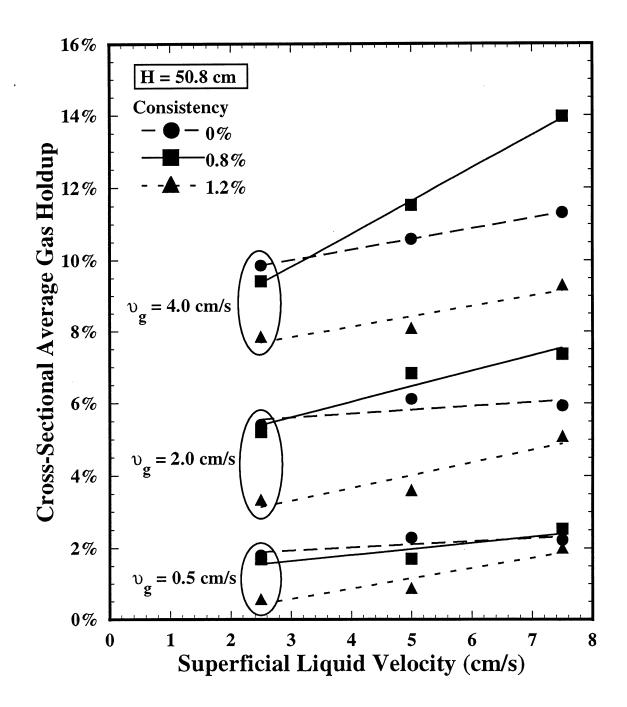
Figure 6: Cross-sectional average gas holdup as a function of superficial liquid velocity at H = 50.8 cm.
