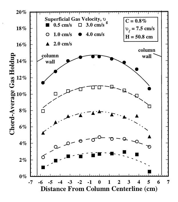
Figure 4: Chord-average gas holdup profiles at various superficial gas velocities for C=0.8%,  $\upsilon_{\ell}=7.5\,$  cm/s, and  $H=50.8\,$  cm.
