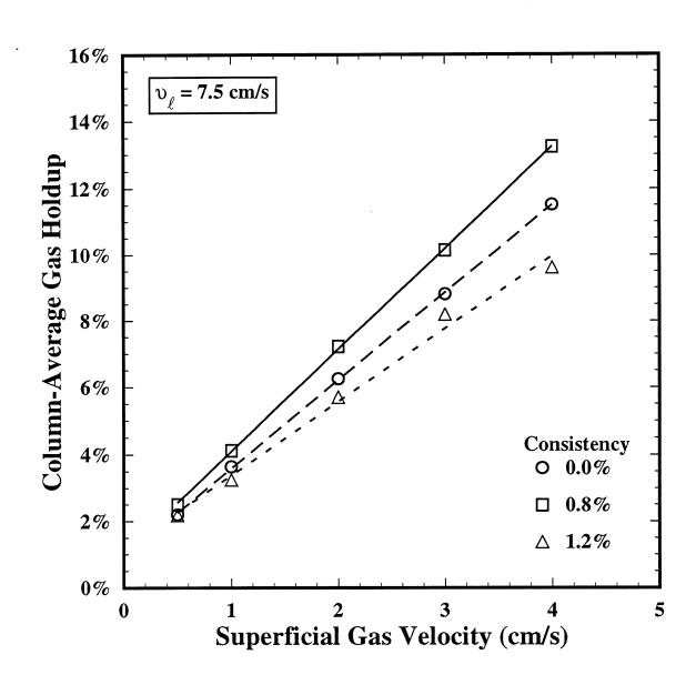
Figure 11: Column-average gas holdup as a function of superficial gas velocity at  $v_{\ell}$  = 7.5 cm/s.
