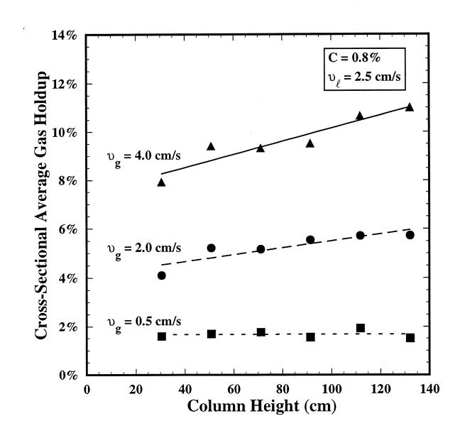
Figure 3: Effect of column height on cross-sectional average gas holdup.
