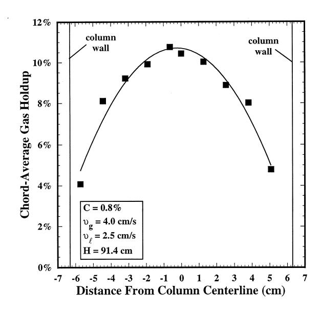
Figure 2: Typical chord-average gas holdup profile.
