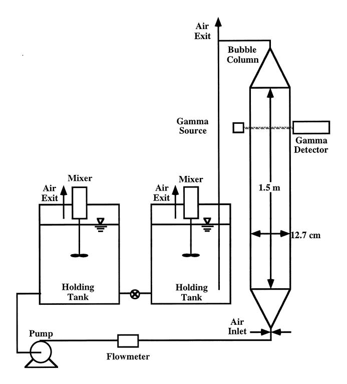
Figure 1: Schematic of the cocurrent bubble column flowloop.
