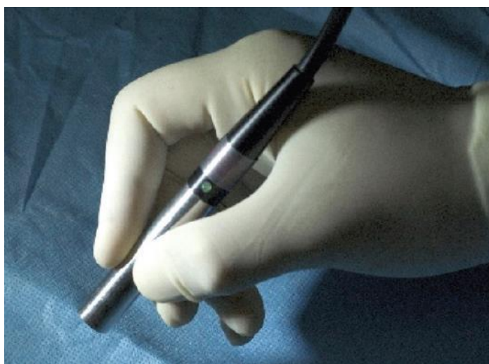
Figure 1.4 – A hand-held spectroscopic device for intraoperative tumor detection. Reprinted from Mohs et al [82] with permission. Copyright © 2010 American Chemical Society.
