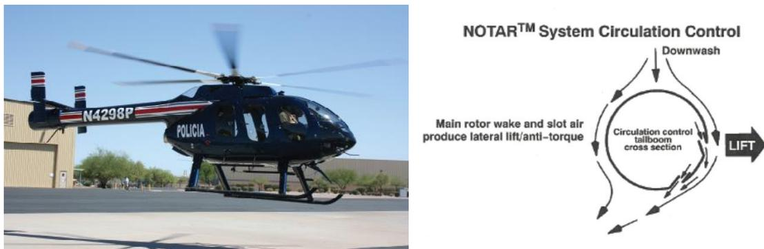
**Figure 2.10. MD600 that utilizes the NOTAR system on the tail boom (left) and cross sectional view of the tail boom (right) (Stephens 2012)**
