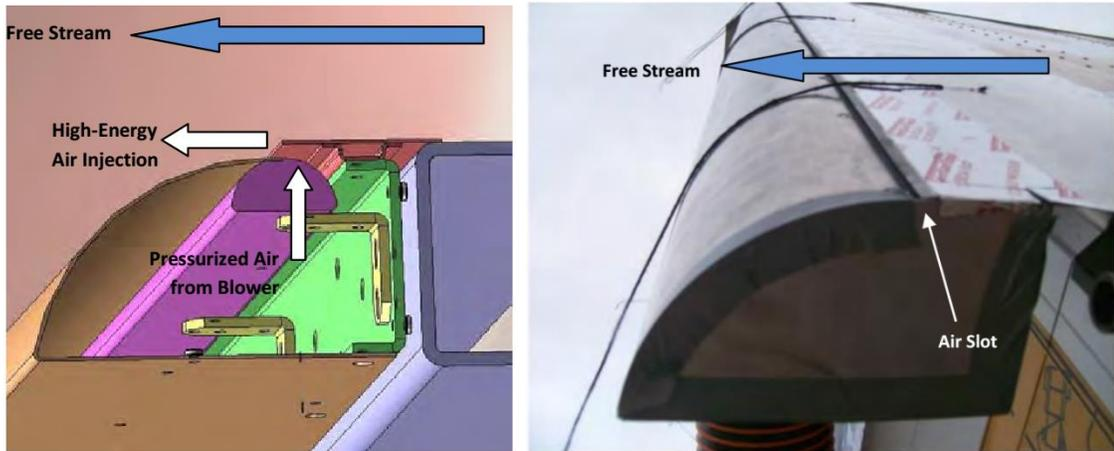
Figure 2.11. Steady AFC system integrated into back of trailer (ATDynamics 2011)
