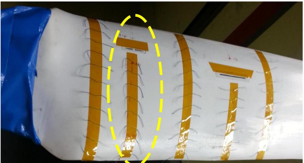
**Figure 2.13. Unsteady AFC device integrated into root of wind turbine blade (Seifert et al. 2015)**
