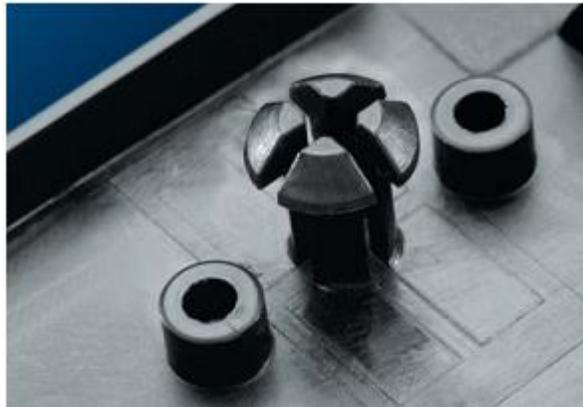
**Figure 4.10. Example of discontinuous annular snap-fit (BASF Corporation 2007)**
