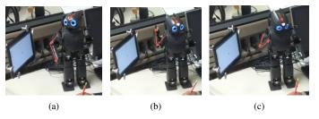
Fig. 3. The fast arm gesture broken down into three parts. (a) Initial Position -Darwin is standing and has eye contact with the tablet-based test. (b) Darwin's right arm is raised, and eye contact is towards the student. (c) Darwin's arm is brought down at a fast speed, and his head follows this downward motion. He then returns to the initial position.
