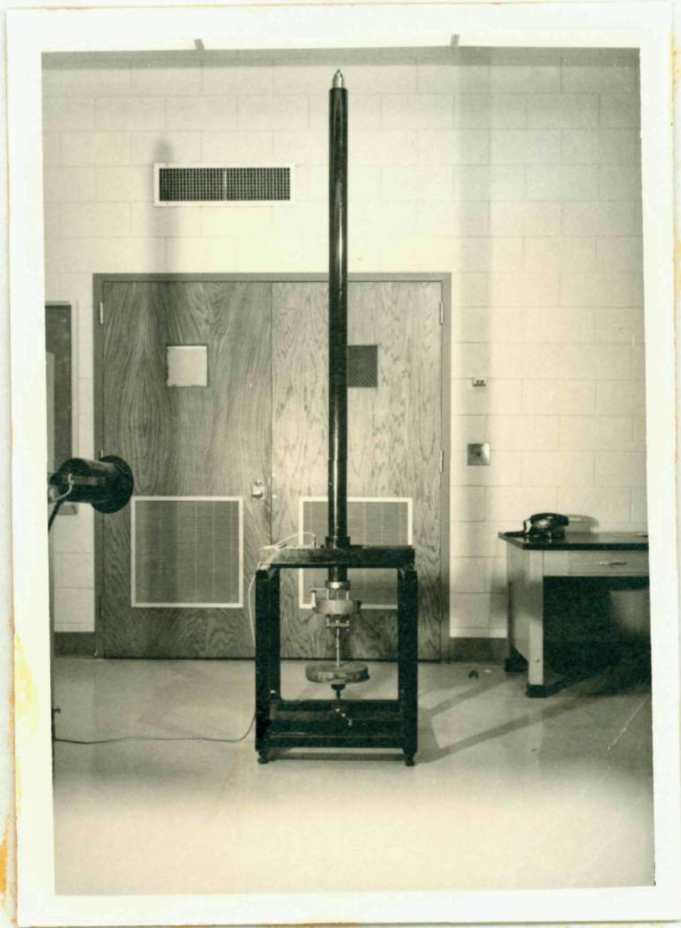
Fig. 2. Photograph of the Creep Test Machine
