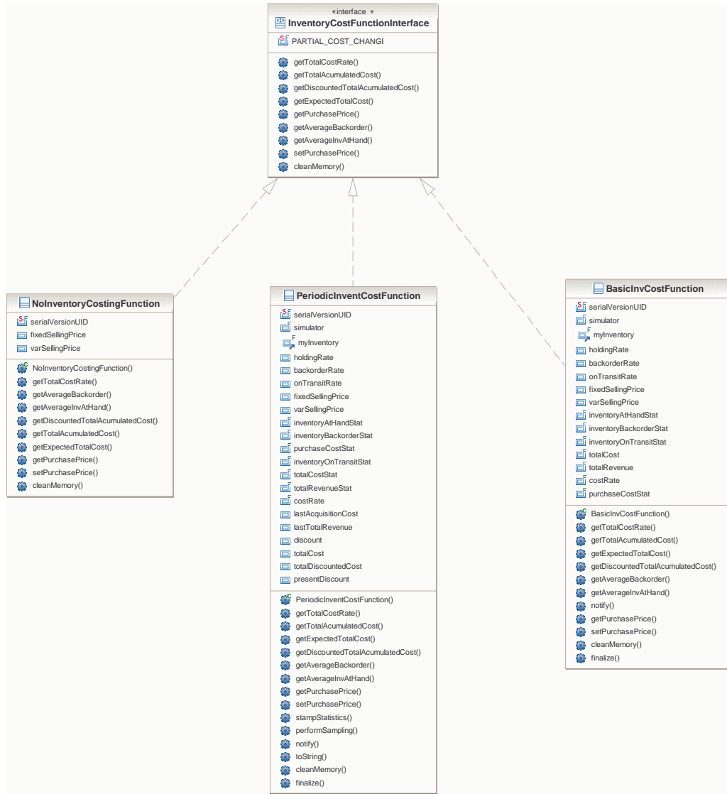
Figure 15: Class Diagram for the Cost Package
