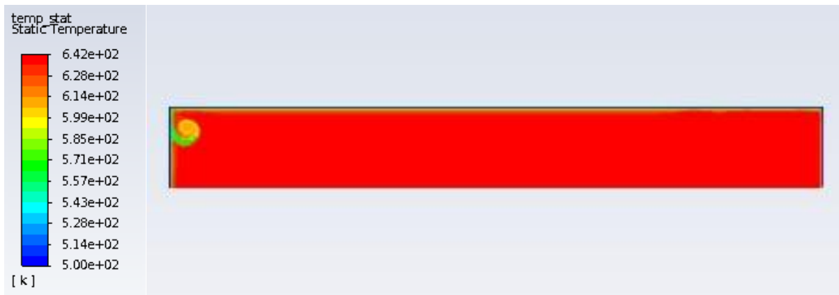
Figure 8: Baseline case through compression, CR = 1.44
