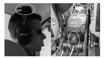
Figure 2: Configuration of orientation tracking device in the headslaved (left panel) and plane-slaved (right panel) conditions of the experiment. In each case, the location of the IMU unit has been circled.
