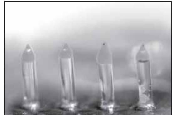
Model drug encapsulated in biodegradable polymer microneedles (height 0.5mm) for controlled release into skin.
