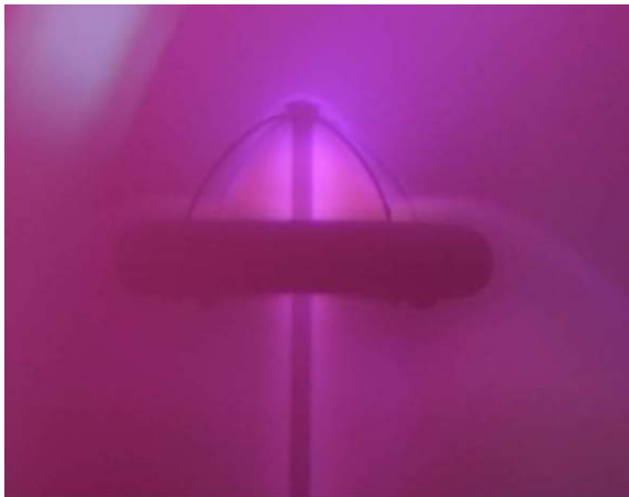
Fig. 6. Mach 12, low density flow over 3-D model of the trailing ballute configuration provides additional CFD model validation data.
