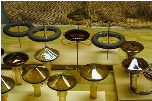
Fig. 4. Several thin film and free flying ballute wind tunnel models of various configurations were constructed and tested at NASA Langley.
