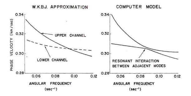
Figure 26. A Detailed Plot of a Section of Fig. 25 Showing a Region of Resonant Interaction Between Two Modes.
