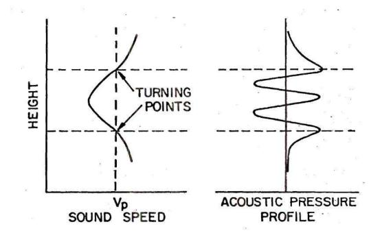
Figure 24. Sketches of Sound Speed and Acoustic Pressure Amplitude Versus Height for a Guided Mode Illustrating the Mechanism of Acoustic Ducting.
