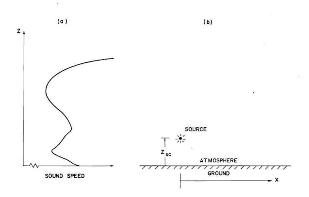
Figure 27. Sketches Illustrating General Propagation Model. (a) Typical Profile of Sound Speed Versus Height. (b) Sketch of Point Source Above a Flat Rigid Ground.
