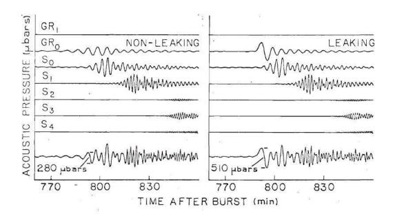
Figure 20. Plots of Modal and Total Waveforms Before and After Inclusion of Leaking Modes (50-Megaton Burst).
