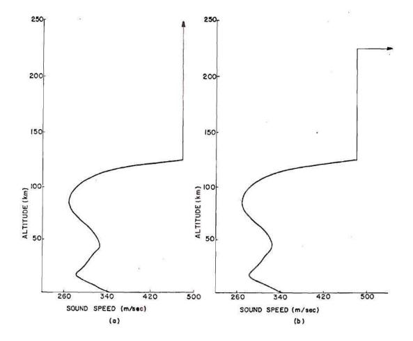
Figure 16. Two Model Atmosphere Profiles. (a) The Same as in Fig. 8. (b) The Same Only with the Original Upper Halfspace Replaced by a Layer of Finite but Large Thickness with a Halfspace Above it of Extremely High Temperature and Sound Speed.
