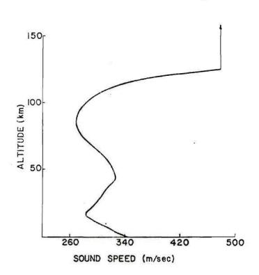
Figure 8. Model Atmosphere Showing Sound Speed Versus Altitude for Numerical Example Treated in the Present Chapter.
