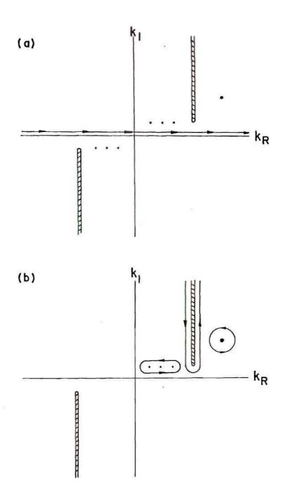
Figure 1. Integration Contours in the Complex k-(Horizontal Wave Number) Plane. (a) Original Contour. (b) Deformed Contour.
