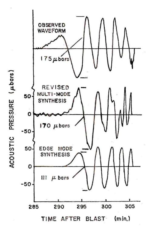
Figure 22. Observed and Theoretical Pressure Waveforms at Berkeley, California, Following the Housatonic Detonation.
