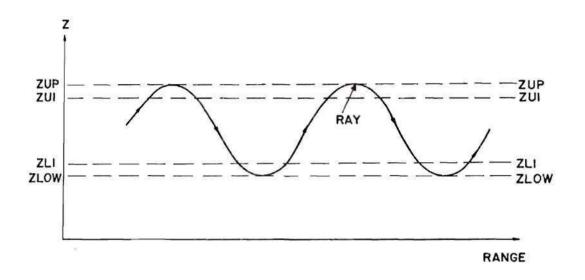
Figure 33. Definition of Parameters ZUI (Slightly Below Upper Turning Point ZUP) and ZLI (Slightly Above Lower Turning Point ZLOW).
