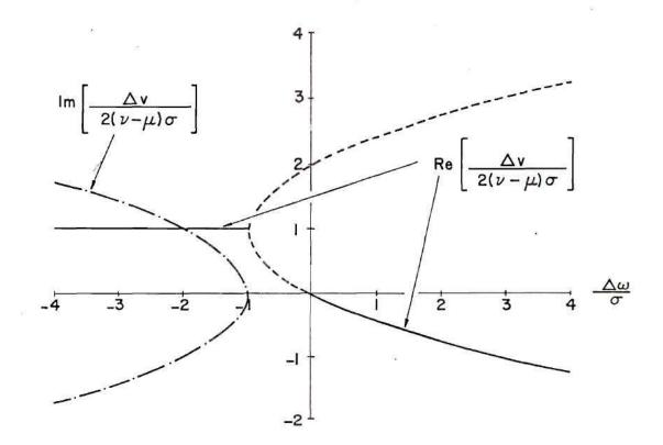
Figure 7. Graph of Normalized Phase Velocity Versus Normalized Frequency in the Vicinity of the Point  $(v_L, \omega_L)$  for the GR<sub>0</sub> Mode.
