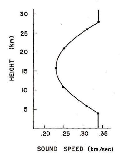
Figure 30. Simplified Hypothetical Sound-Speed Profile with Lattice Points Shown.
