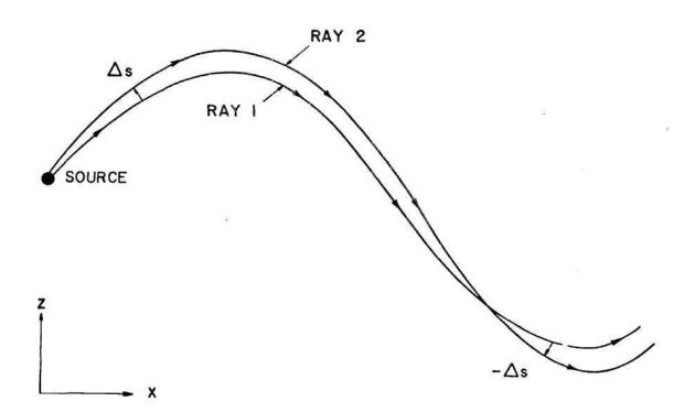
Figure 32. Definition of Parameter  $\Delta s$  Which Characterizes Two Adjacent Rays with Horizontal Phase Velocities  $v_{p1}$  and  $v_{p2}$ .
