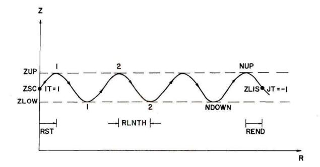
Figure 31. Parameters for Characterizing a Ray.
