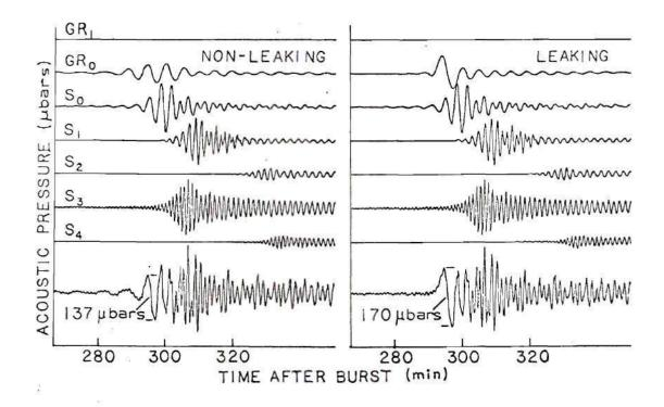
Figure 21. Plots of Modal and Total Waveforms Before and After the Inclusion of Leaking Modes (Housatonic).
