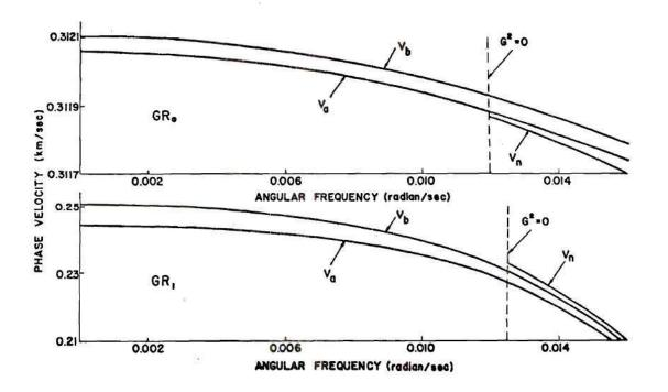
Figure 4. Curves of Phase Velocity  $(v_n, v_a, v_b)$  Versus Angular Frequency  $(\omega)$ .
