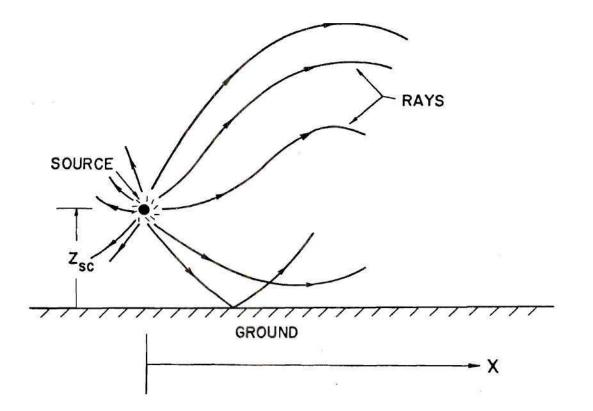
Figure 28. Sketch of Acoustic Rays Emanating from a Source in an Atmosphere in Which the Sound Speed Varies with Height.
