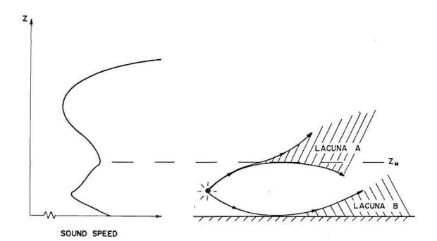
Figure 29. Examples of the Occurrence of Lacunae in the Propagation of Rays from a Source in a Stratified Atmosphere.
