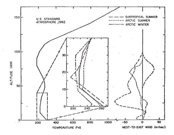
Figure 23. Profiles of Temperature and Wind Speed Versus Height for Standard Reference Atmospheres.
