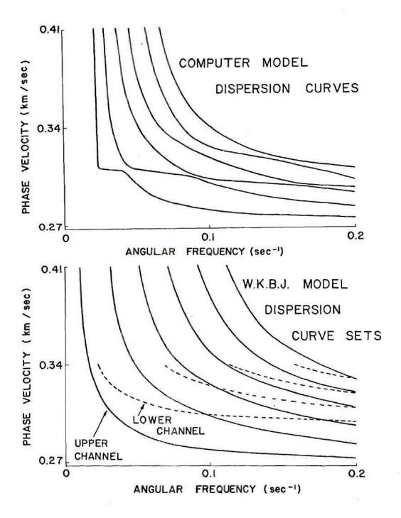
Figure 25. A Comparison of Theoretical Guided-Mode Dispersion Curves for the U. S. Standard Atmosphere, 1962.
