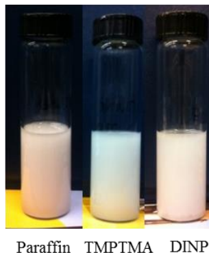
Figure 2.7 Attempts of producing foam via frothing in the presence of secondary liquids only (14.16 wt. %).
