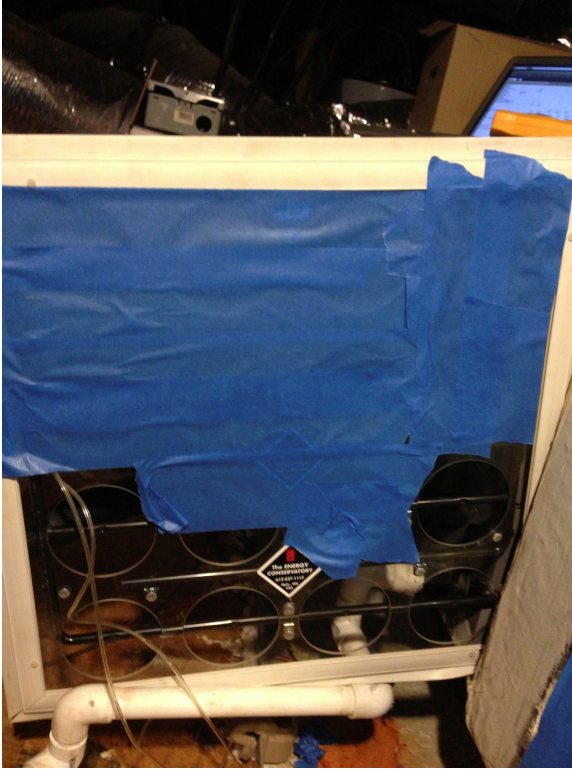
Figure 10. An example of a partially taped filter (“TrueFlow Taped 3”).
