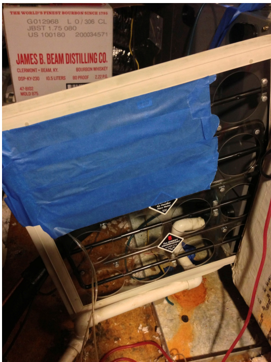
Figure 9. An example of a partially taped filter (“TrueFlow Taped 2”).
