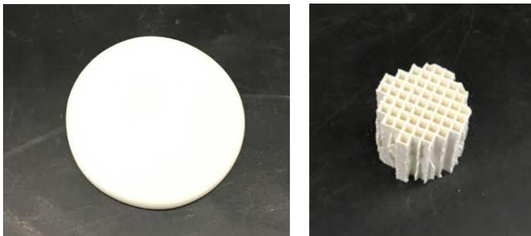
Figure B.1 Flat \alpha -alumina support (left) in plate form used for X-ray diffraction analysis of the \text{Mg}_2(\text{dobpdc}) and the 100 CPSI cordierite monolith wash-coated with \alpha -alumina (right) used to grow \text{Mg}_2(\text{dobpdc}) functionalized with mmen.
