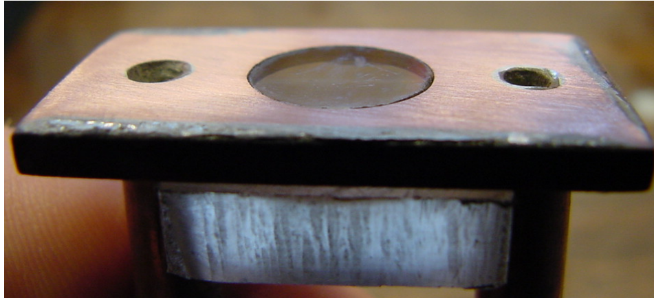
Figure 8: Backside of polycarbonate and copper cover plate.
