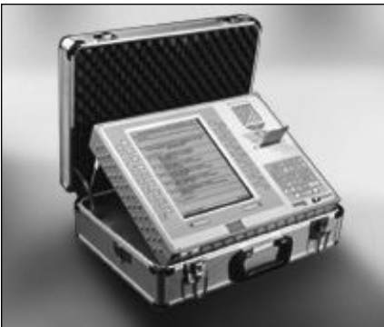
Selected residents of Decatur and Lithonia participated in November’s Direct Record Electronic (DRE) Voting Systems Pilot Project, which tested this machine built by Diversified Dynamics (above). Instead of paper ballots, voters receive a “smart card” that acts like an ATM card, unlocking the terminal for vote casting.
