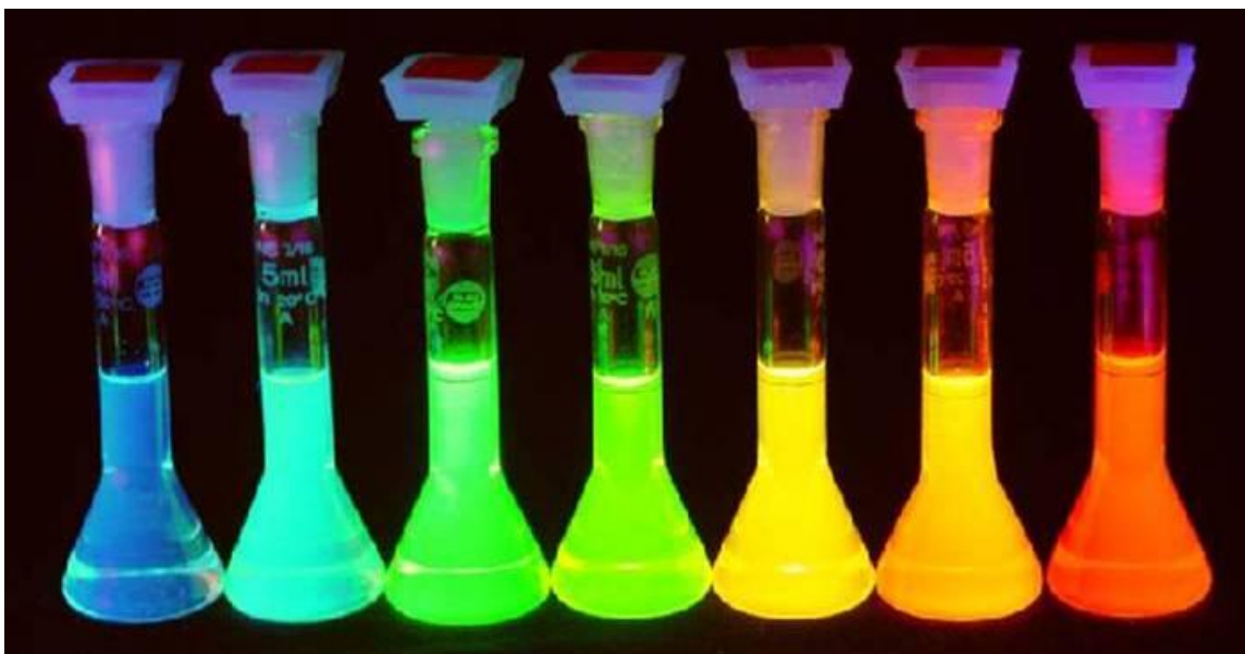
Figure 1.4 These vials contain solutions with different sized monodispersed CdSe quantum dots. On the left is the smaller, sized quantum dots, ranging from blue to red.
