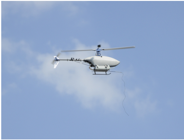
(a) The 2lbs AFI Hornet Micro utilizes a MaxStream Wireless Serial Link and an Analog Video Transmitter
