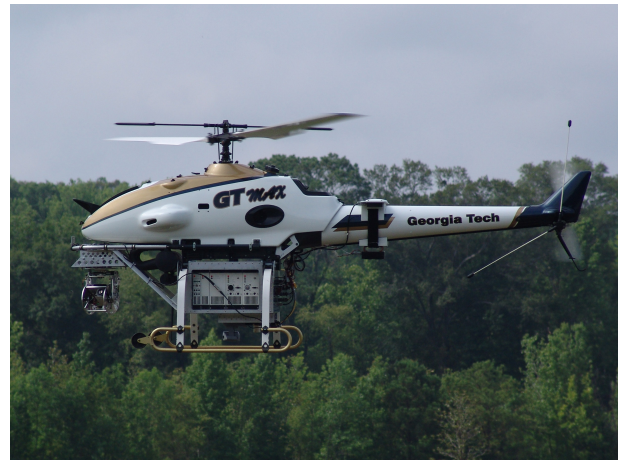
(b) The 160lbs GTMax Research UAV utilizes 802.11b/g, FreeWave Wireless Serial Links, and an Analog Video Transmitter
