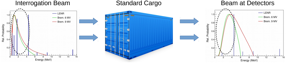
Figure 2.1: Work-flow of a cargo scanning system from a radiation detection standpoint. The left shows the energy distribution of various interrogation beams and the right shows the energy distribution of those beams after penetration through the container. The black circle highlights the differences in the low-energy end of the spectrum. These photons are preferentially absorbed in the cargo container, imparting dose while not contributing to image quality. The LENR beam is relatively robust to this effect since it has a higher-energy, discrete distribution.
