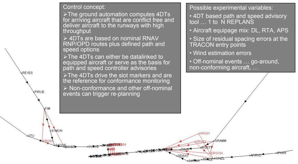
Goal: A control strategy that enables quiet, fuel efficient Optimized Profile Descent operations with high throughput and is robust to disturbances and off-nominal events while keeping aircraft on RNAV routes.
