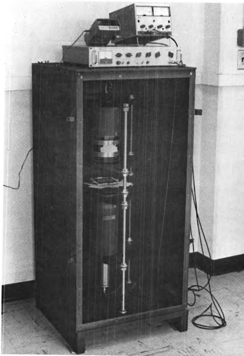
Figure 15. Photograph of apparatus for optical measurement of fiber alignment.
