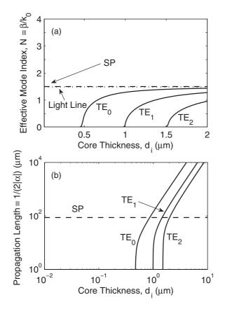
FIG. 3. (a) Effective mode indices N and (b) propagation lengths L for the  $TE_{0-2}$  modes as functions of  $d_i$  in MIM (Au-SiO<sub>2</sub>-Au) waveguides at  $\lambda = 1550$  nm. The curves for the MIM  $TE_{0-2}$  modes and the single Au/SiO<sub>2</sub> interface are labeled  $TE_{0-2}$  and SP, respectively.
