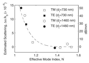
FIG. 10. Estimated scattering attenuations for the TM and TE modes based on the  $\Delta \alpha / k_0$  column in Table II. The general trend is shown by the dashed curve.
