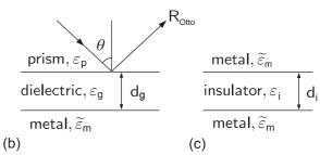
FIG. 4. (a) Schematic diagram of the ATR configuration applied to a symmetric MIM structure. The transmission matrix corresponding to each numbered layer is labeled. (b) A single metal/dielectric interface (Otto configuration, Ref. 17). (c) A symmetric MIM structure.
