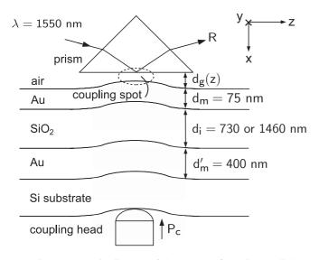
FIG. 5. Schematic diagram of the ATR configuration applied to the MIM structures.
