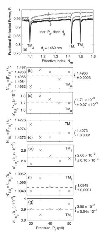
FIG. 8. (a) TM reflectance angular spectra for the structure in Fig. 5 with  $d_i = 1460$  nm measured at various  $P_c$ . (b)  $N'_{TM_0}$  and (c)  $\alpha'_{TM_0}/k_0$  of the TM<sub>0</sub> resonances. (d)  $N'_{TM_1}$  and (e)  $\alpha'_{TM_1}/k_0$  of the TM<sub>1</sub> resonances. (f)  $N'_{TM_2}$  and (e)  $\alpha'_{TM_2}/k_0$  of the TM<sub>2</sub> resonances.
