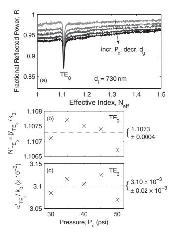
FIG. 7. (a) TE reflectance angular spectra for the structure in Fig. 5 with  $d_i = 730$  nm measured at various  $P_c$  values. (b)  $N'_{\text{TE}_0}$  and (c)  $\alpha'_{\text{TE}_0}/k_0$  of the TE<sub>0</sub> mode.
