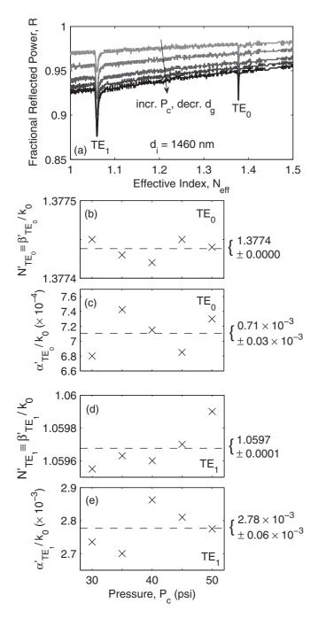
FIG. 9. (a) TE reflectance angular spectra for the structure in Fig. 5 with  $d_i = 1460 \text{ nm}$  measured at various  $P_c$  values. (b)  $N'_{\text{TE}_0}$  and (c)  $\alpha'_{\text{TE}_0}/k_0$  of the TE<sub>0</sub> resonances. (d)  $N'_{\text{TE}_1}$  and (e)  $\alpha'_{\text{TE}_1}/k_0$  of the TE<sub>1</sub> resonances.
