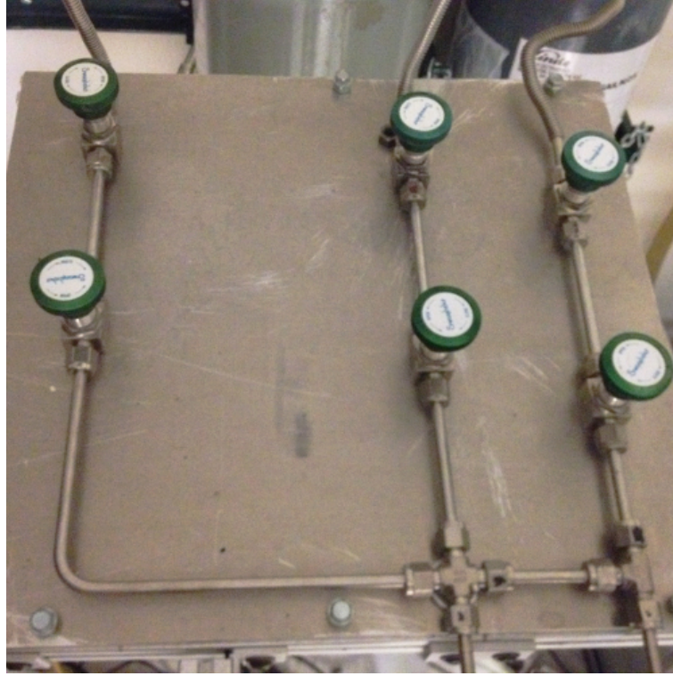
Figure 2.8: Gasline system. Three lines connect to three different gas cylinders (on the back, not shown) and each line has two Swagelok valves. Two lines in front, one is connected to a turbo pump and one is hooked up to the growth chamber via a leak valve.
