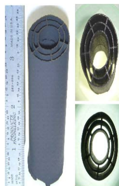
Fig. 6. LCA with good straightness and roundness. Two interior circumferential cracks can be seen in the top right photo and there is one small interior longitudinal crack that is not visible in the photo.
