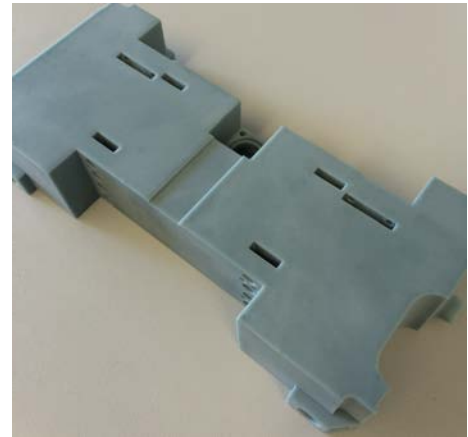
Fig. 2 The 3D-printed structure of the BioSentinel thruster, with no other components attached.
