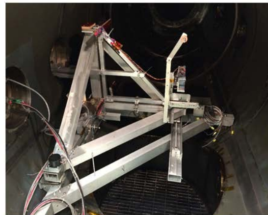
Fig. 4 The BioSentinel thruster mounted to the test stand in the vacuum chamber at Georgia Tech (left) and at the NASA Glenn Research Center (right).
