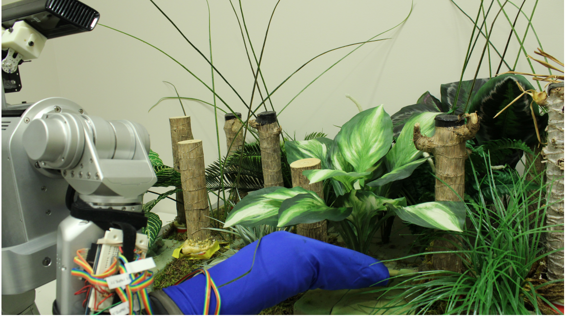
Figure 11: A robot DARCI, equipped with a tactile-sensing sleeve (blue) and a Kinect, reaching into the cluttered foliage environment.
